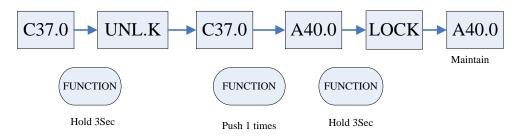
**C.** To display Chamber Temperature, hold FUNCTION for 3 seconds + push FUNCTION once after 5 seconds. Chamber Temperature will switch back to the lowest temperature between Chamber and Airway Temperatures.
