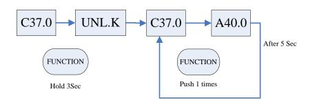
B. To maintain Airway Temperature on the display, hold FUNCTION for 3 seconds + push FUNCTION once
