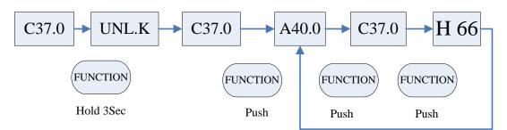
**A.** To display Airway Temperature, hold **FUNCTION** for 3 seconds + push **FUNCTION** once after 5 seconds.
