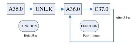
**D.** To maintain Chamber Temperature on the display, hold FUNCTION for 3 seconds + push FUNCTION once+ hold FUNCTION for 3 seconds.
