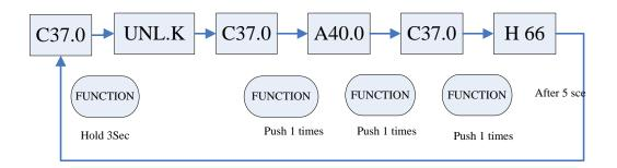
**F.** To maintain on Heater Plate Temperature on the display, hold **FUNCTION** for 3 seconds + push **FUNCTION** 3 times + hold **FUNCTION** for 3 seconds.
