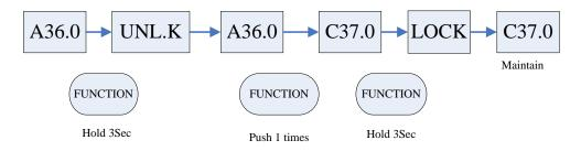
**E.** To display Heater Plate Temperature, hold **FUNCTION** for 3 seconds + push **FUNCTION** 3 times. Heater Plate temperature will display for 5 seconds and switch back to the lowest temperature between Chamber and Airway temperatures.
