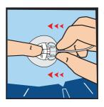
Place a finger on the cannula housing while pushing the site connector straight in until you hear a "click".
